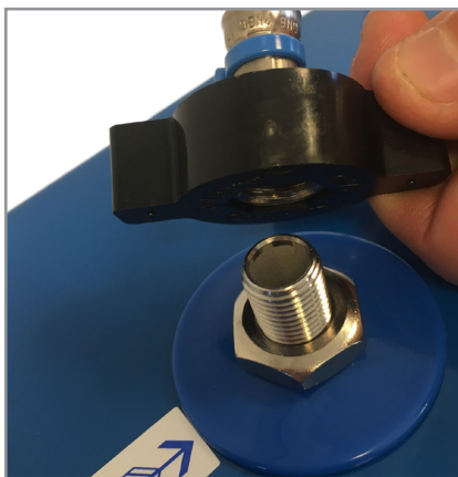
Attaching the water outlet hose (blue)
